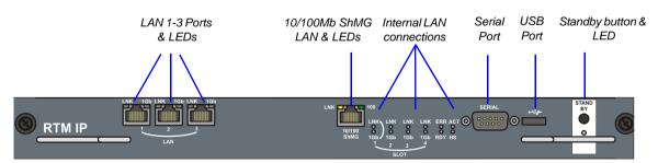
LAN1, LAN 3, ShMG and the Serial ports are only for debugging and not for customer use
